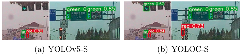
Fig. 10. Traffic light detection results on the S 2 TLD dataset. YOLOC-S reduces missed detections.
